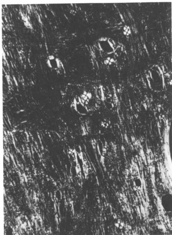
Fig. 5. Polarizing light microscopy of hydrated (> 70 wt.% water) bovine brain sulfatide at 70°C. A neat phase mosaic texture with oily streaks and focal conics is observed.
